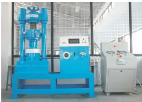
UKL Gasket Test Laboratory showing machines for testing compressibility, recovery and sealability.
