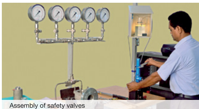
Assembly of safety valves
