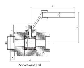
Screwed/ Socket-weld end - Class 1500
